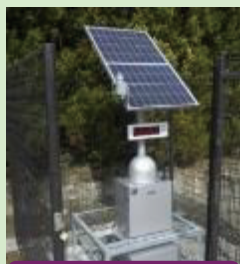
Transportable type Monitoring Post
